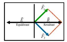
The resultant of two or more forces (vectors) is found by balancing the forces with another force (weights on a hanger) so that the ring is centered
