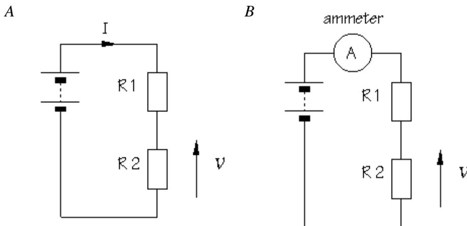
**to measure current, the circuit must be broken to allow the ammeter to be connected in series**
