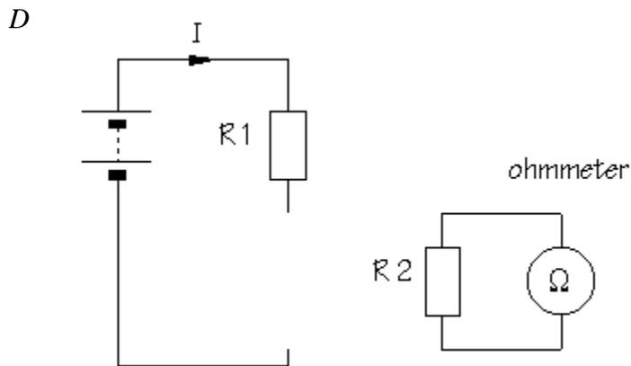
**to measure resistance, the component must be removed from the circuit altogether**
