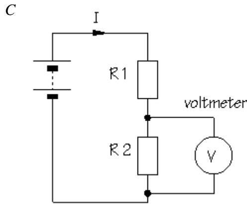
**to measure potential difference (voltage), the circuit is not changed:
